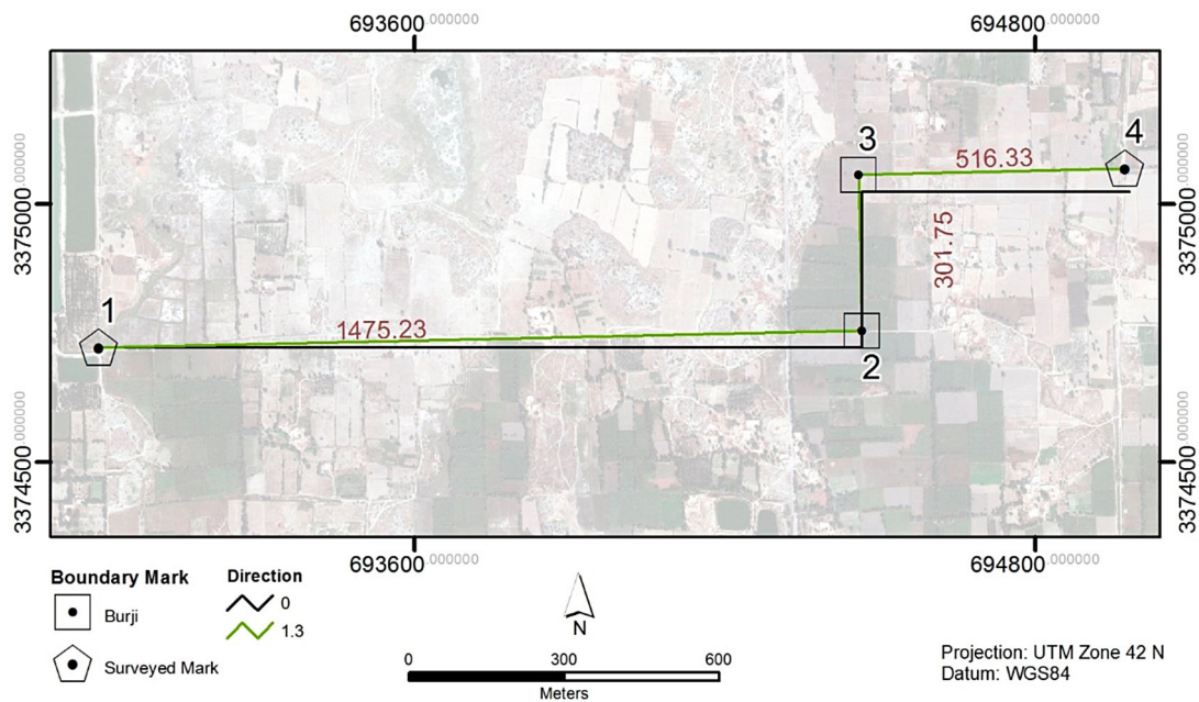
5 Connecting boundary marks using actual lengths and computed directional shift
