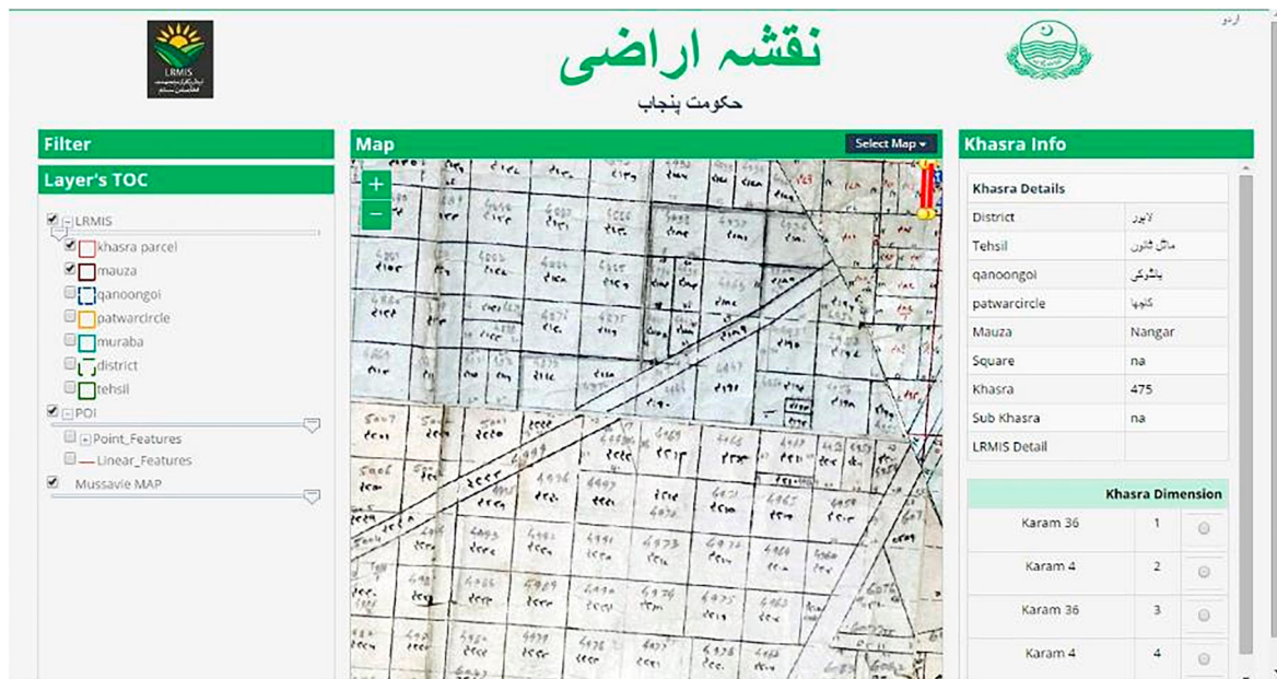
A: Skewness and mismatch in paper-based cadastral maps in Lahore district (Source: http://lrma.punjab-zameen.gov.pk/ ).
