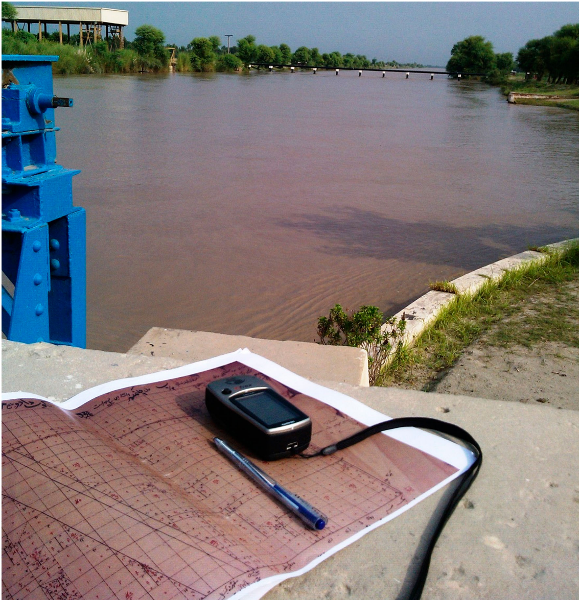
C: Garmin eTrex handheld GPS receiver for boundary marks survey.
