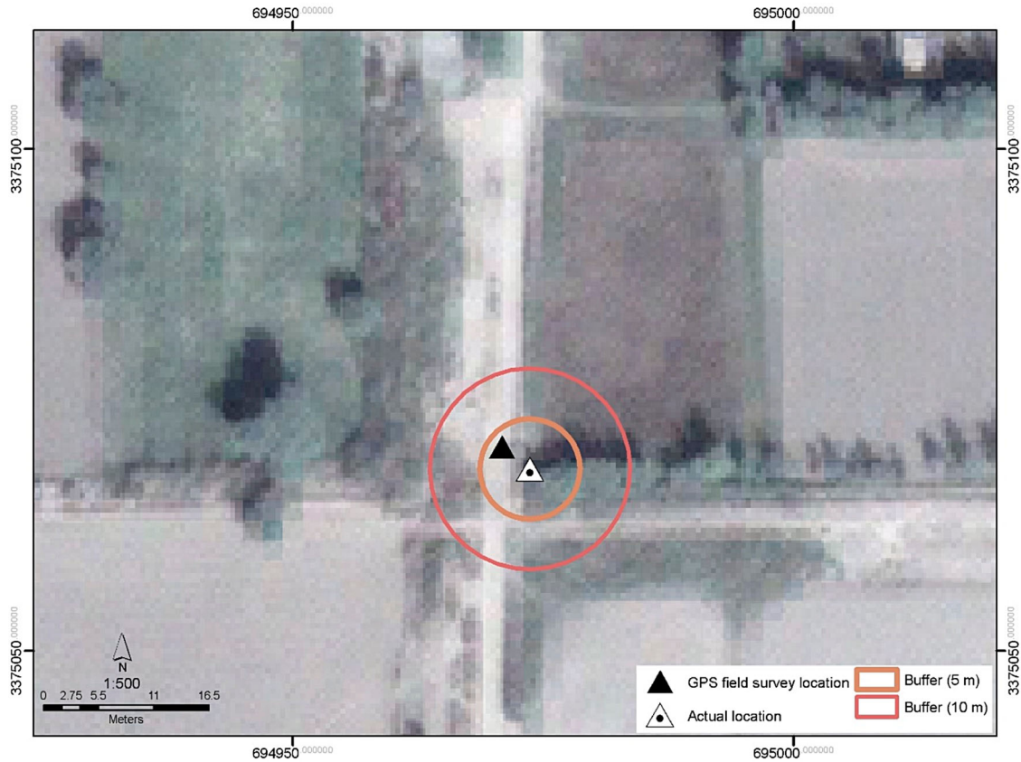
4 The displacement between the actual and GPS field survey location of boundary mark on satellite imagery. Courtesy of the DigitalGlobe Foundation
