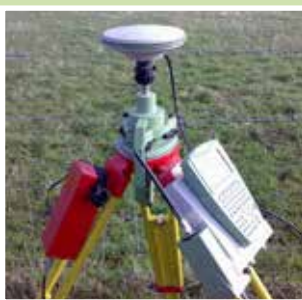
Temporary reference station on a geodetic reference point
